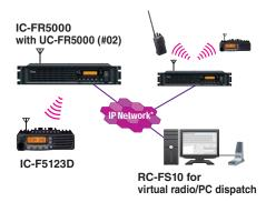
When using the IC-F5123D series in IDAS multi-site conventional mode, the IC-F5123D can communicate with other IDAS radio users working with other repeater sites and/or virtual radio/PC dispatch stations on the IDAS network.
