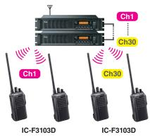
The IC-F3103D series can be used in an IDAS single-site trunking system.
