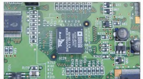
Circuit board with ANALOG DEVICES A/D converter chip
