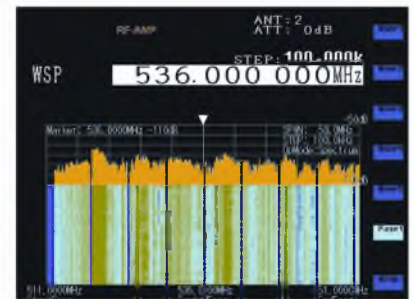
Digital TV broadcast signal (in Japan, center freq. 536MHz)
