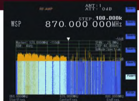
WSP 870.000000 MHz (displays 1GHz of BW on the LCD)
